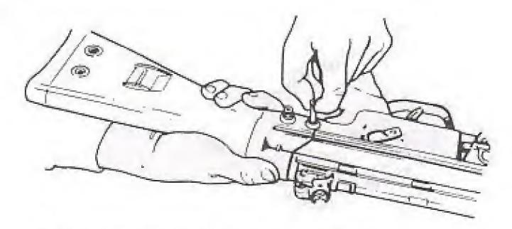
3. Remove the two takedown pins located just forward of the stock. No tools should be required to push the pins through from the right side to the left side of the rifle. When the pins are removed, they should be stored in the small storage holes in the rear of the stock.
